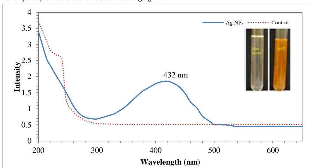
Figure 2: UV-Vis absorption spectrum of (a) *Emih sonchifoha* plant extract and biosynthesized SNPs (visual observation during reduction process (inset))
