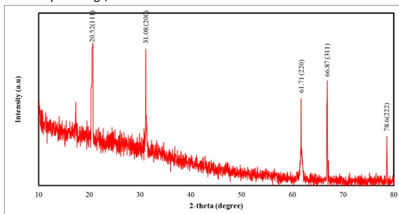
Figure 4: XRD patterns of Ag nanoparticles.
