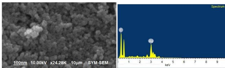
Figure 5: SEM image of silver nanoparticles synthesised using *Emih sonchifoha* plant extract and EDX spectrum of synthesised SNPs (right)
