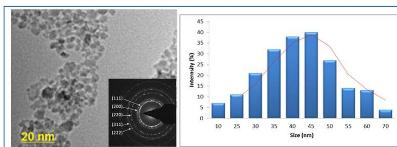
Figure 6: TEM micrographs showing spherical silver nanoparticles, and the SAED pattern and particle size distribution showing most of the particles in the size range of 30-50 nm (Right side image)
