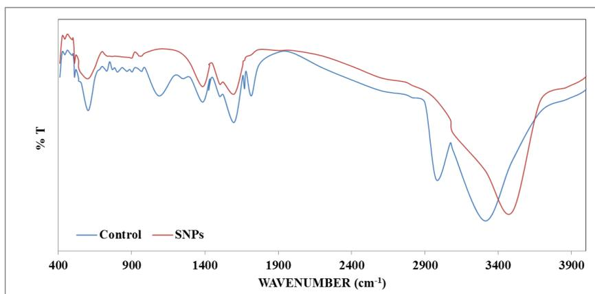
Figure 3: FTIR spectra of plant extract and synthesized silver nanoparticles
