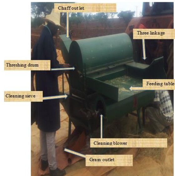
Figure1. Major parts of modified tractor operated Bako Teff thresher
