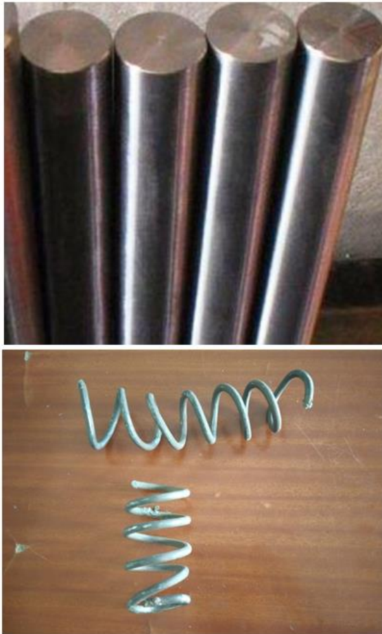
Figure 1 : Shaft and spring specimens before heat treatment.
