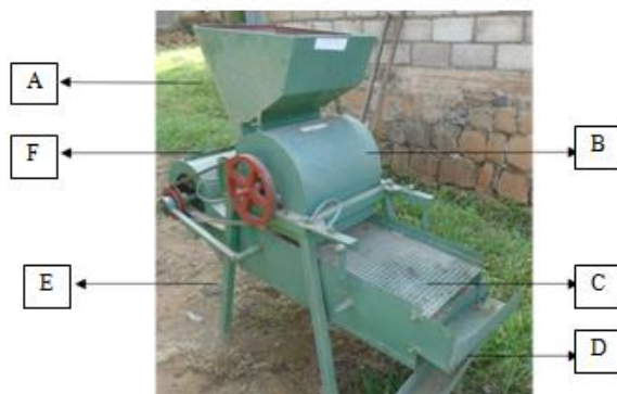
Figure 1. The pictorial picture of the sheller. A – Hopper, B – Drum unit, C – Sieve, D – Delivery unit, E – Frame, F – Fan
