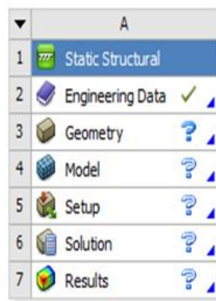
Figure4. Step by step procedure of propeller Blade Analysis in ANSYS.
