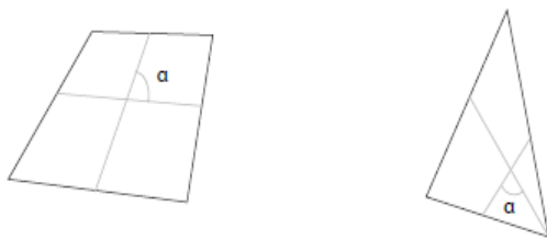
Fig.3.Skew in Mesh quality.
