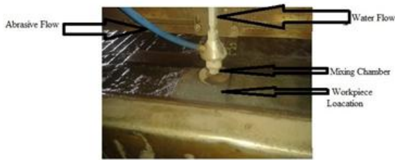
Fig. 1. Abrasive Water Jet Machining of Inconel-825
