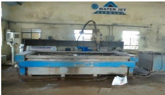
Fig.4. Excel Abrasive water Jet Machine Set up
