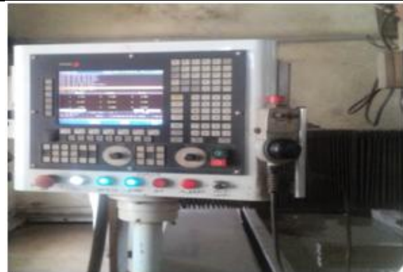
Fig.5. Control Panel for Abrasive water jet Machine
