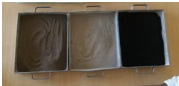
Fig 4 : Samples of black cotton soil, flyash and crumb rubber
