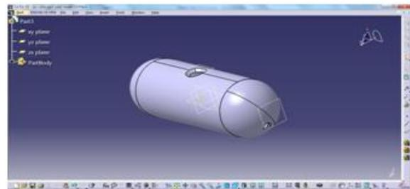
Fig. 3 Pressure vessel model in CATIA Software by contains radius of 25mm
