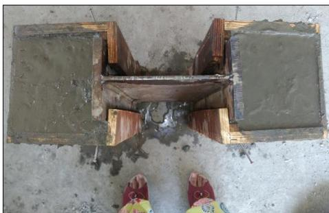
FIG.-8 CASTING OF PUSH-OUT SPECIMEN
