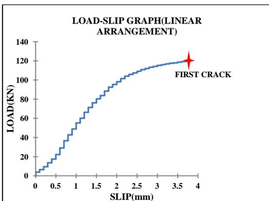
**FIG-14 LOAD-SLIP BEHAVIOR OF LINEAR ARRANGEMENTS OF STUDS**
