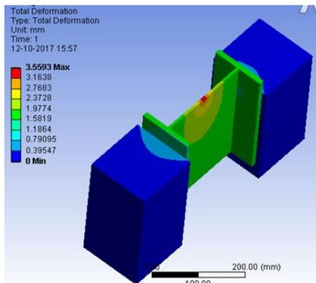
FIG-3: TOTAL DEFORMATION OF SINGLE STUD (PUSH-OUT MODEL)
