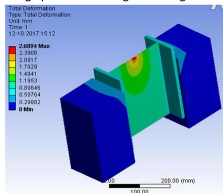
FIG-4: TOTAL DEFORMATION OF SQUARE ARRANGEMENT OF STUDS (PUSH-OUT MODEL)
