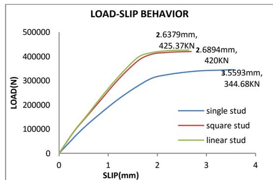
FIG-6: COMPARISON CHART OF ANALYTICAL RESULTS OF SINGLE & MULTI-STUD SHEAR CONNECTORS
