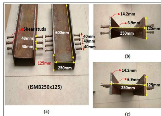
**FIG-7 (A) STUD TYPE CONNECTION (B) SQUARE ARRANGEMENT (C) LINEAR ARRANGEMENT**
