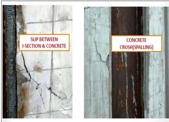
**FIG-10 FAILURE MODE ON CONCRETE**
