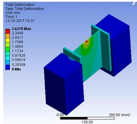
FIG-5: TOTAL DEFORMATION OF LINEAR ARRANGEMENT OF STUDS (PUSH-OUT MODEL)
