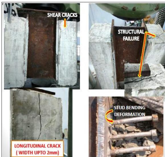
**FIG-11 CRACKS DUE TO FAILURE AND STUD DEFORMATION**
