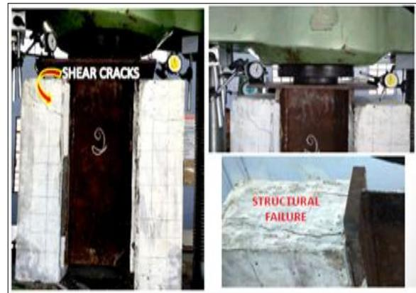
**FIG-12 CRACKS DUE TO FAILURE**
