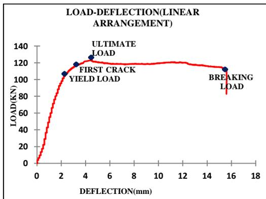
**FIG-13 LOAD-DEFLECTION BEHAVIOR OF LINEAR ARRANGEMENTS OF STUDS**
