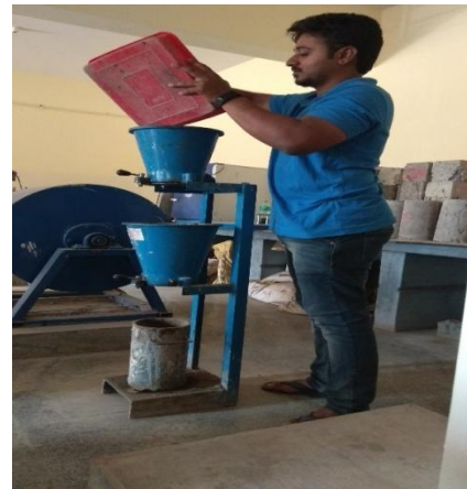
Fig 3.2: Compaction factor test
