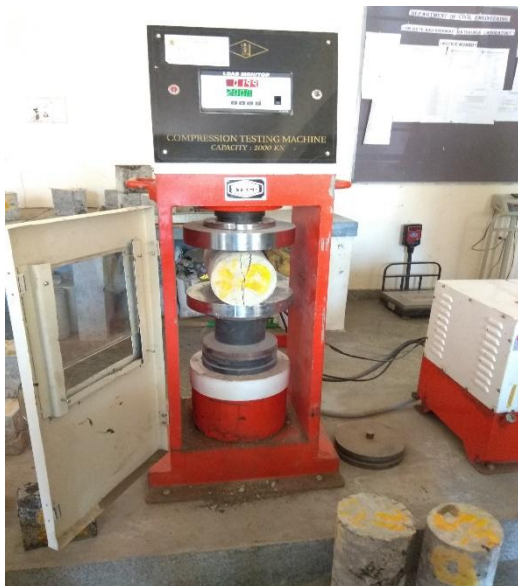
Fig 4.2: Split tensile test
