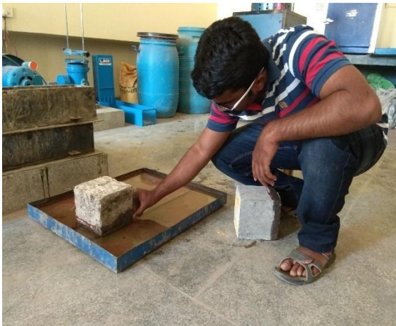
Fig 5.4: Measuring height of water after 24 hrs.
