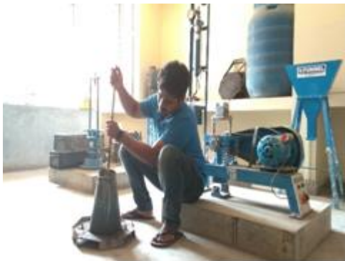
Fig 3: Slump cone test
