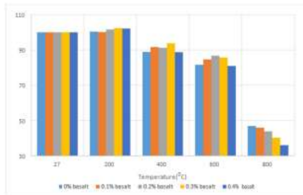
Fig. 4.6: Variation of % residual compressive strength with temperature for plain concrete and concrete with 0.1, 0.2, 0.3 and 0.4% basalt fibers (28 days)
