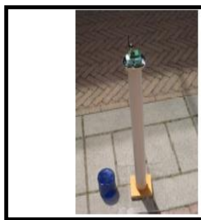
Figure 6: An optical beacon used as a navigation
