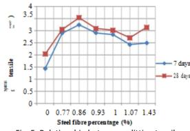
Fig. 5. Relationship between splitting tensile strength (fct) and steel fibre percentage (%)
