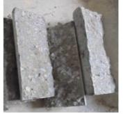
Fig. 10 Failure of plain concrete Cylinder
