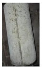
Fig. 11 Failure of SFRC Cylinder CONCLUSIONS AND RECOMMENDATIONS
