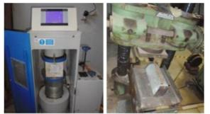
Fig. 2. Digital compression Fig. 3. Splitting tensile testing testing machine
