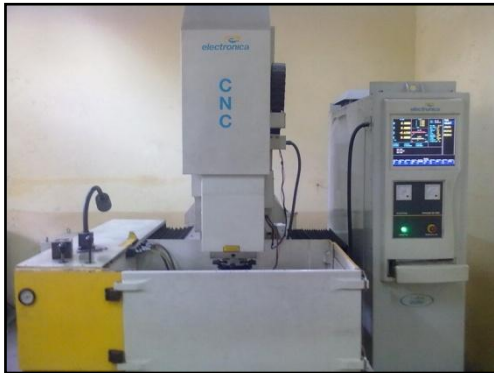
Figure 3.1 CNC die sinking EDM (Model: xpert-1, Make: Electronica Machine Tool, India)
