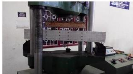
Fig -7: Flexural Load setup
