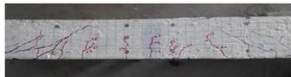
Fig -8: Crack pattern for control beam
