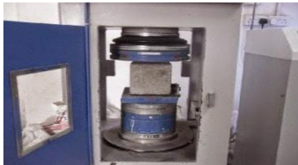
Fig.6:Compression test of cement
