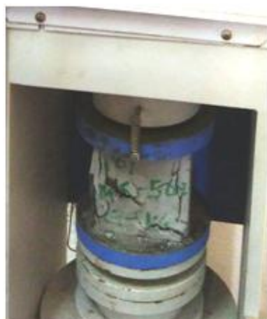
Fig. Cube after failure in compressive testing machine
