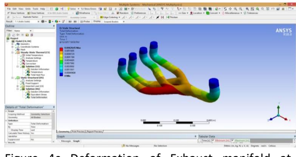
Figure 4c Deformation of Exhaust manifold at 1000°C
