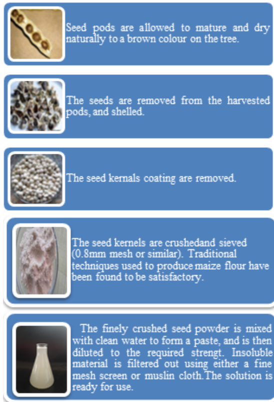
Fig4 : Flow chart of preparation of Moringa oleifera coagulant
