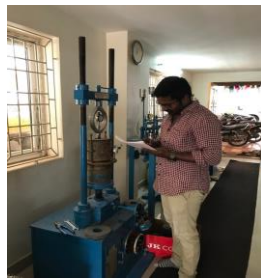
Fig 9: Performing CBR test in the laboratory
