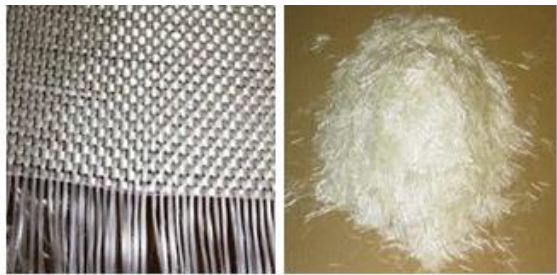
Fig : 3 Glass fibre (geotextile material)
