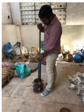
Fig 4: performing heavy compaction
