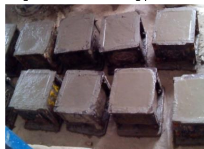
Fig -5: Sampling of Concrete
