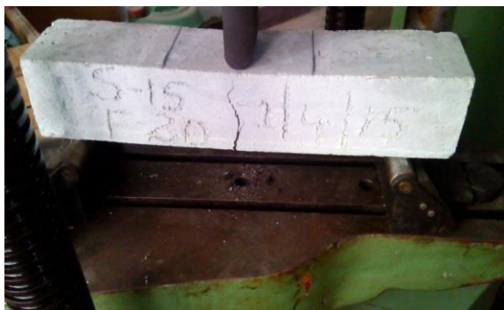
Fig -9: Flex strength test on beam
