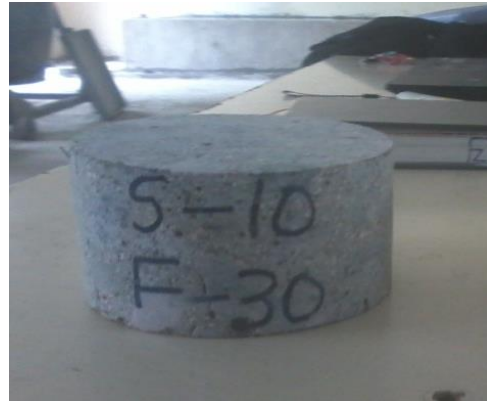
Fig -10: Concrete Specimen with Water absorption Test
