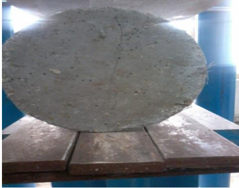
Fig -8: Split Tensile test on Cylinder
