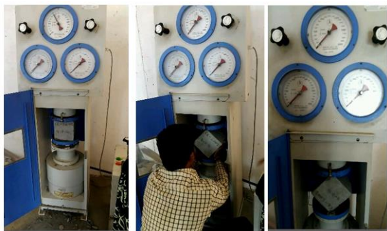
Fig 2: Compressive Strength Test (Left) & Split Tensile Strength Test (Middle & Right)
