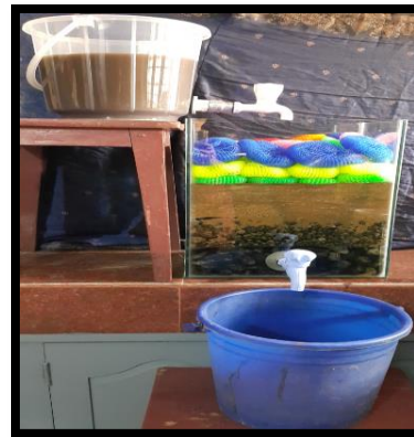
Fig 1. Set up of Filtration Tank
