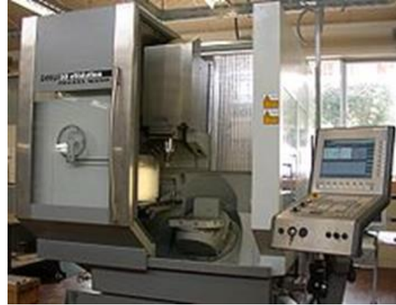
Fig. 2; Five-axis machining center with rotating table and computer interface [4]
