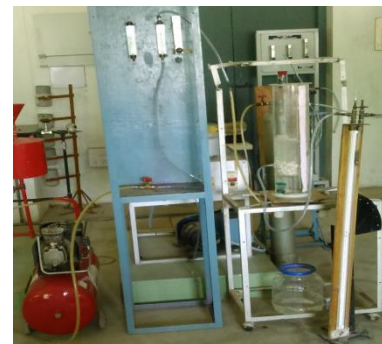
Figure. 2.2 Snapshots of a split cylinder sparged reactor and its parts
