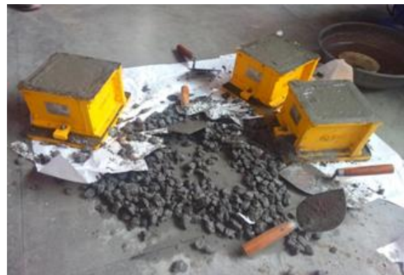
Figure 4. Concrete cube prepared for testing
