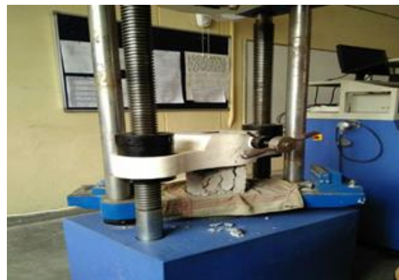
Figure 5. Testing of concrete cube on UTM
