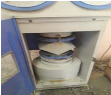
Fig specimen under split tensile strength
