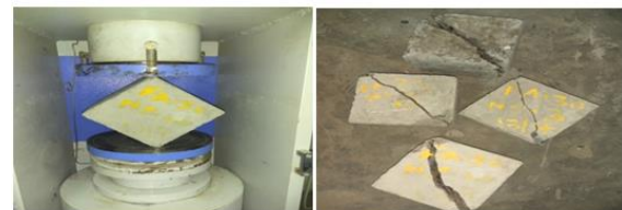
Fig: Split Tensile Strength Test
