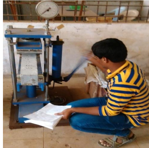
Beam under Shear Test
