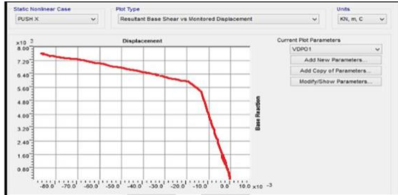
Pushover Curve for Basic Structure
