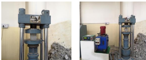
Figure 5: Compression strength and Split Tensile Strength Testing Machines.
