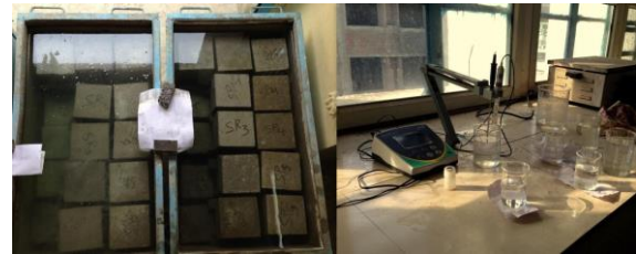
Figure 6: Cubes kept in acid and alkalinity solution and apparatus for measuring pH of solution (pH meter).
