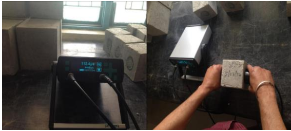
Figure 7: Cubes UPV Test Apparatus
