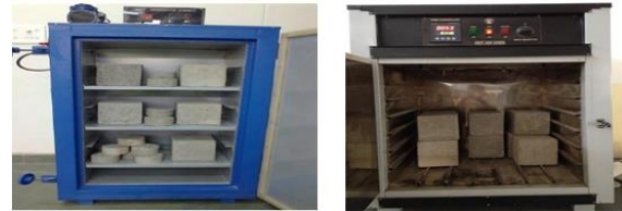
Figure 8: Conditioning and drying of samples in desiccator and oven respectively
