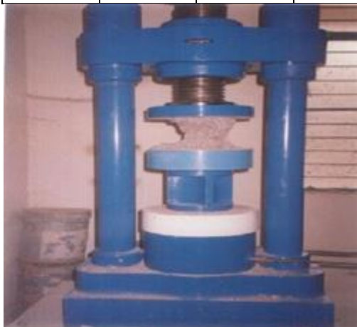
Fig -3: Typical Fracture Pattern of Cube Specimens due to Compression Load
