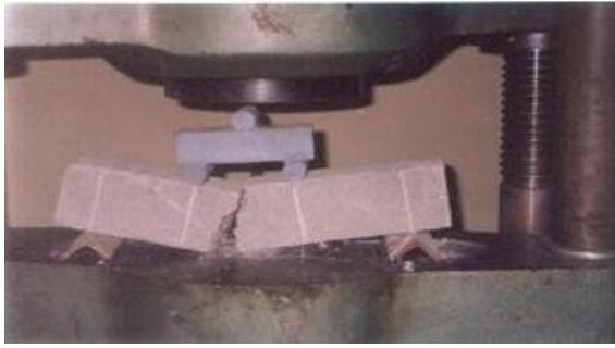
Fig -4: Typical Fracture Pattern Of Bea Specimens due to flexural Load-M30,0% Fly ash.
