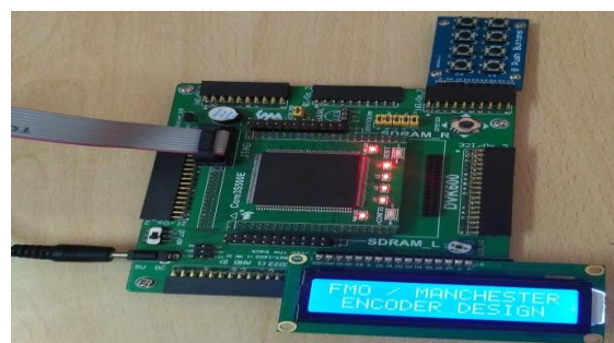
Fig.13: FM0-Manchester - Reset Mode Display The hardware based design simulation is performed
