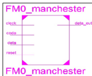
Fig 9: Block diagram of FM0/Manchester Encoder
