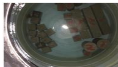
Curing of concrete specimens
