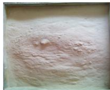
Fig -1: Sample of Flyash going to mixed in Concrete
