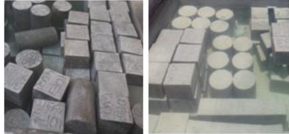
Fig -6: figure shows a curing tank in which concrete specimens were kept for 3,7,28,56,90 days for hydrating of concrete.
