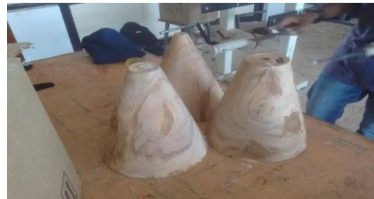
Fig. 1 Wooden patterns 15°, 18° and 21°
