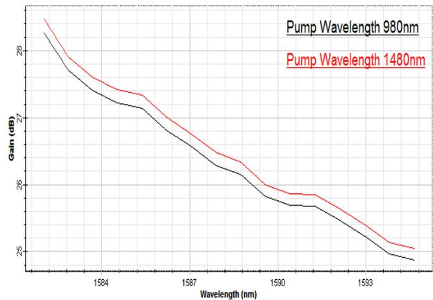
Figure3. Gain vs Wavelength
