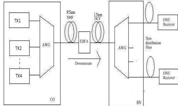
Figure 1: Block Diagram of Simulation Setup
