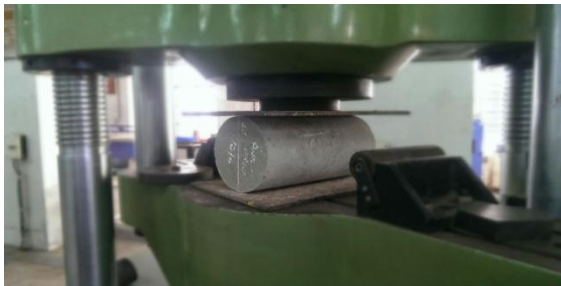
Fig. 6 Split Tensile Strength test
