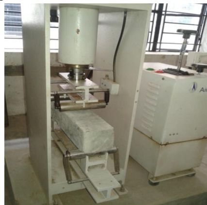
Fig. 5 Flexural Strength test
