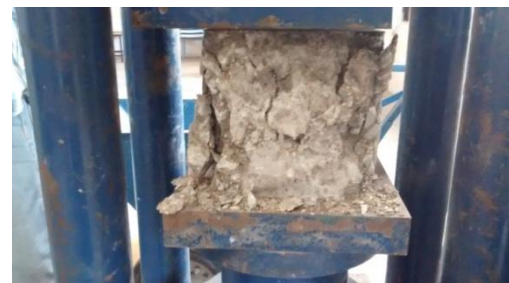
Figure 5. Compression Failure of cube
