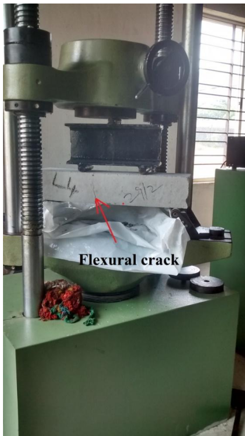
Figure 6. Beam flexural test
