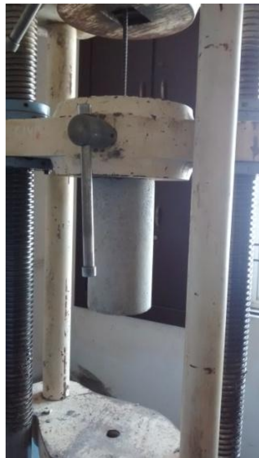
Figure 7. Bond strength set up
