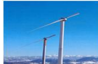
Fig 2.5.5 Single blade HAWT
