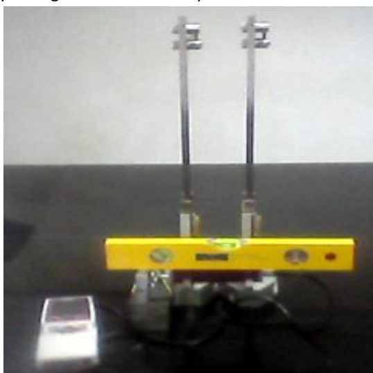
Figure 2: Leveling of SR Probe
