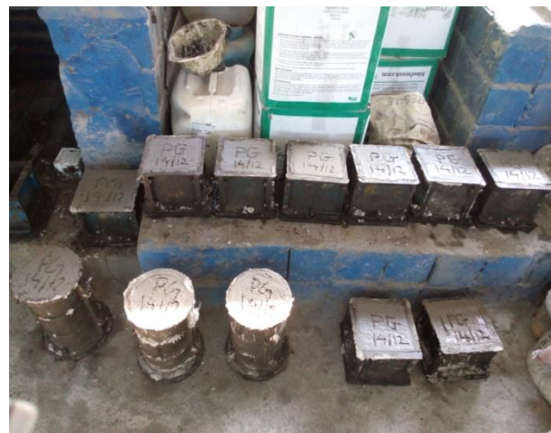
Fig No. 4.1 Identification marks has been marked after casting
