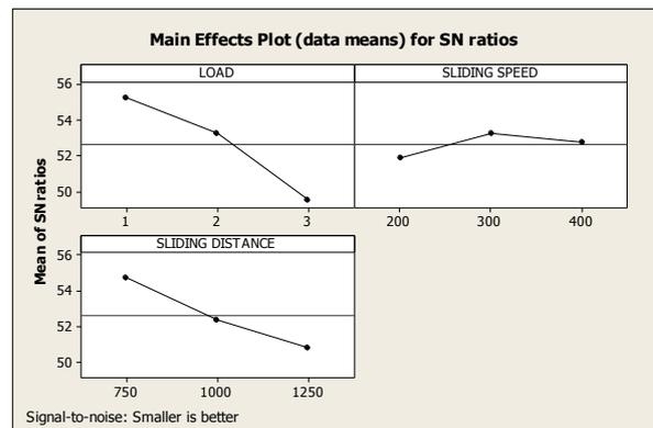
**Fig 2.**Main effects plot for S/N ratio-wear
