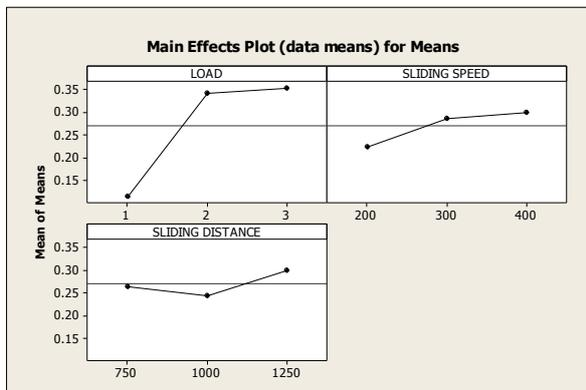
Fig 3. Main effects plot for means-COF
