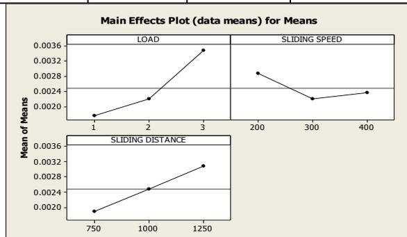
**Fig 1.**Main effects plot for means-wear.
