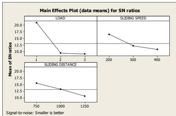
Fig 4. Main effects plot for S/N ratio- COF
