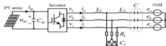
Fig.4. Circuit diagram of a three-phase grid-connected PV inverter with blocking capacitors.
