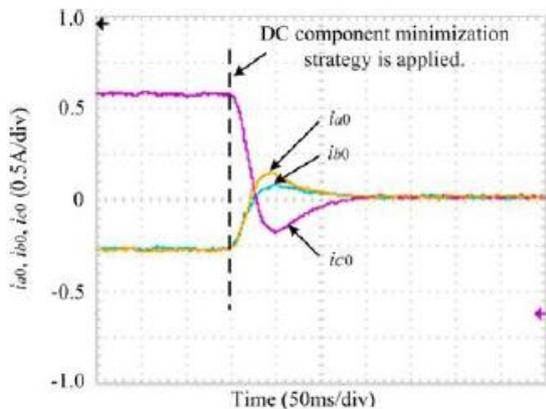
Fig.7(a). Transient response when proposed dc component minimization is applied.
