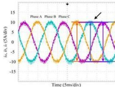
Fig.6. (a) three phase grid current with proposed system with dc component minimization
