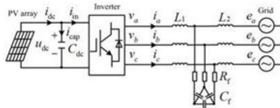
Fig.1 Transformerless three-phase PV inverter system.
