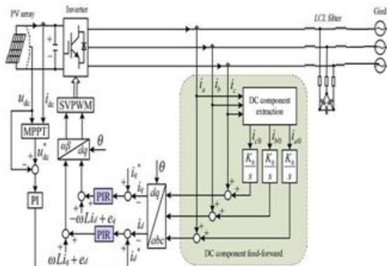
Fig.5 .DC component minimization strategy based on dc component feed-forward and PIR controllers.
