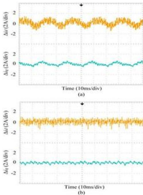
Fig.8. Steady state errors of d-axis and q-axis current with (a) PI controller (b) PIR controller
