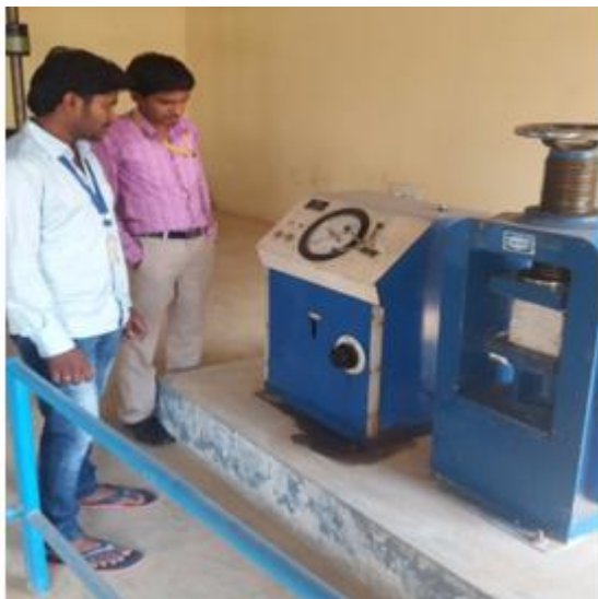
Fig. Compression Test on Cubes
