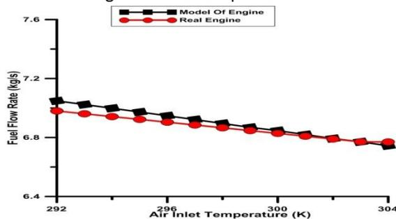
Fig.11ACC with respect to Fuel Flow Rate.
