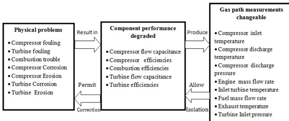
Fig. 2 GT performance degradation scheme.
