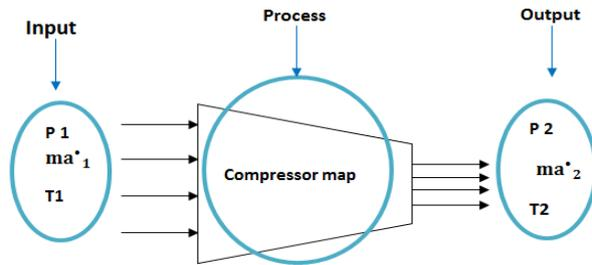
Fig. 4 Compressor process .
