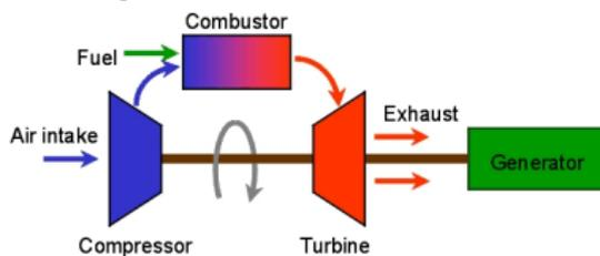
Fig. 1 Gas Turbine Engine.
