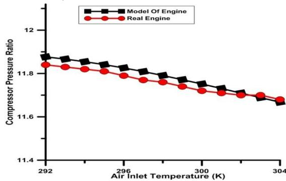
Fig. 9 ACC with respect to Compressor Pressure Ratio.
