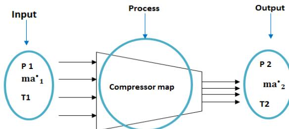
Fig. 4 Compressor process .
