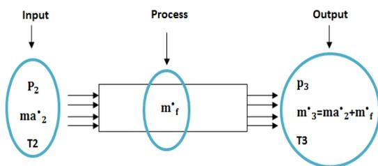
Fig. 5 Combustion chamber process.
