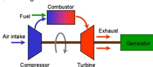
Fig. 1Gas Turbine Engine.
