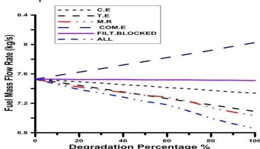
Fig. 17DG with respect to fuel mass flow rate.
