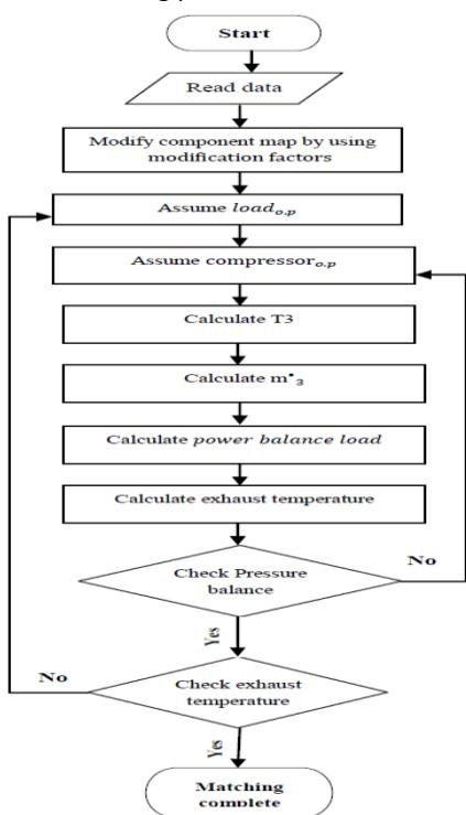
Fig. 7 Correct matching point flow chart
