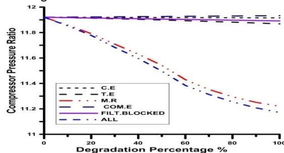
Fig.15DG with respect to compressor pressure ratio.
