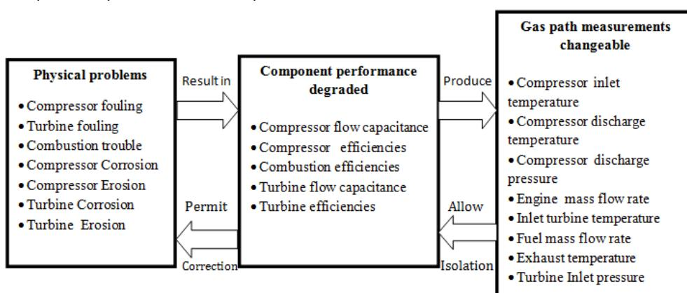
Fig. 2 GT performance degradation scheme.
