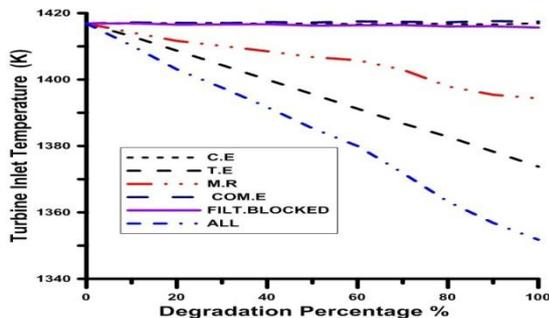
Fig. 16DG with respect to turbine inlet temperature.
