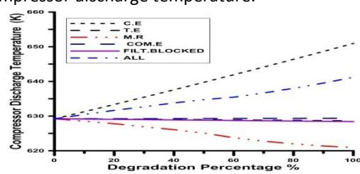
Fig. 14DG with respect to compressor discharge temperature.
