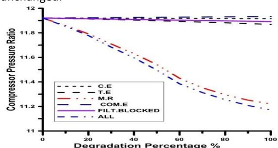
Fig.15DG with respect to compressor pressure ratio. Fig.16 shows how the degradation performance of the engine components affects on the inlet turbine temperature. In which, increase the degradation performance of ( $ALL$ ) leads to decrease of
