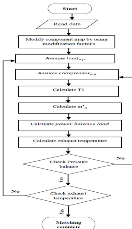
Fig. 7 Correct matching point flow chart
