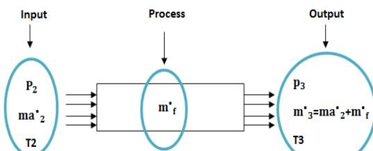
Fig. 5 Combustion chamber process.
