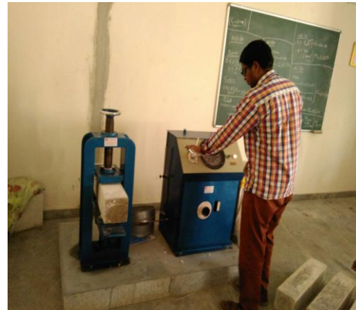
Fig. Flexural test on beams
