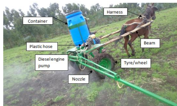
Figure 1. Developed sprayer being tested on the field and its major parts
