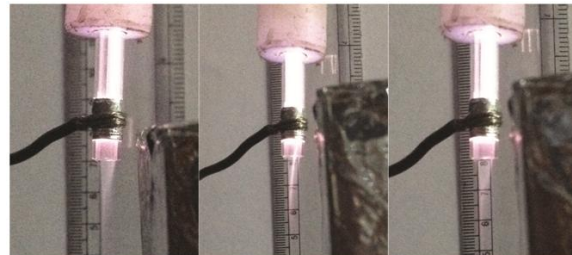
Fig 7: Effect of variation of flowrate (1, 2, 4 ltr/min) at 5kV 0.5cm distance between nozzle and floating electrode
